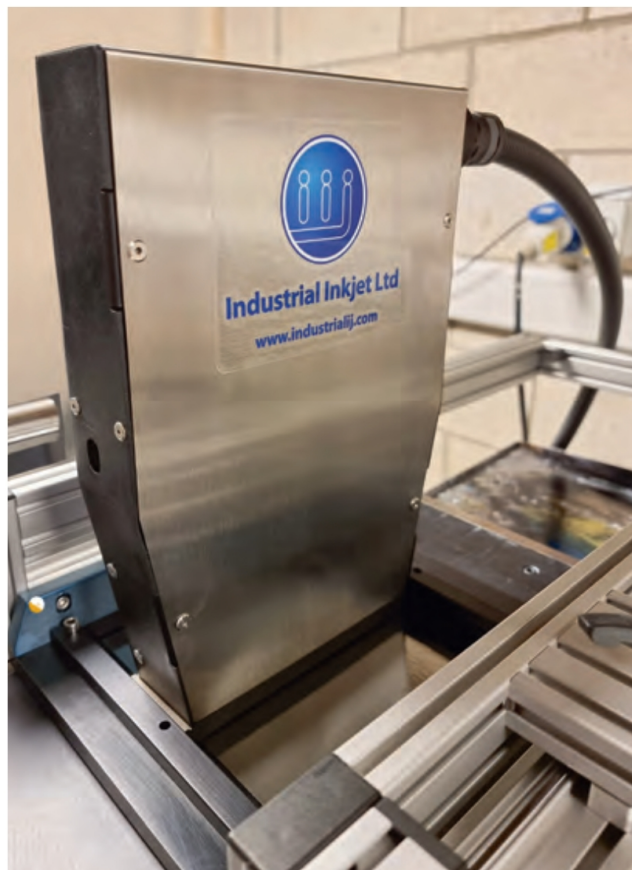
360dpi and 600dpi options, and 72mm or 75mm (pictured) print widths were required for the final machine design
